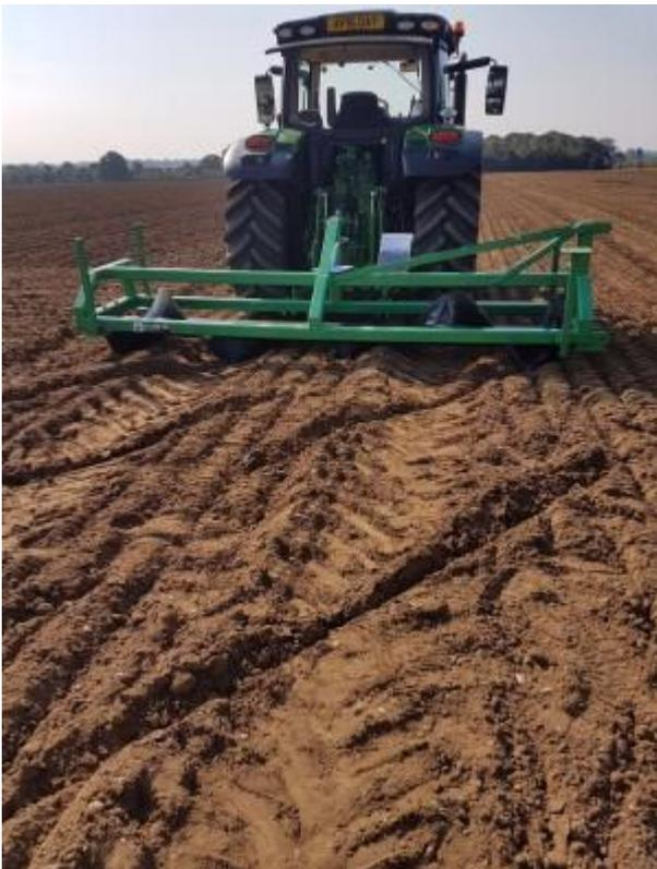
The Earthwake has corkscrew blades, drawn along the ground like a roller, which cut diagonal drainage channels across the tramlines every two metres, dispersing the accumulation of water into areas where it can drain more freely.
